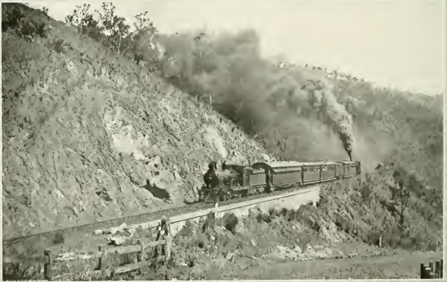
Australia has railroads in assorted sizes—wide, standard, and narrow gauge. This road up Mt. Morgan is a standard gauge, but it has three rails. The middle rail is cogged and it is used both for tractive power, as the engines toil up the steep grades, and for braking, when the train is coming down the mountain.
