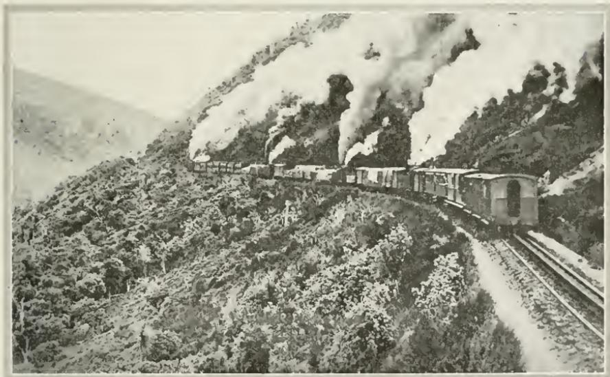
Pulling up what is said to be the steepest railroad grade in the world, over the Rimutaka Mountains, where for three miles the tracks drop one foot in every fifteen. Special locomotives, with steel shoes to grip a center rail as a brake, are used to handle trains on these grades. Terrific winds sweep these mountains, and windbreaks are built to protect the trains. On two occasions trains have been blown from the tracks.
